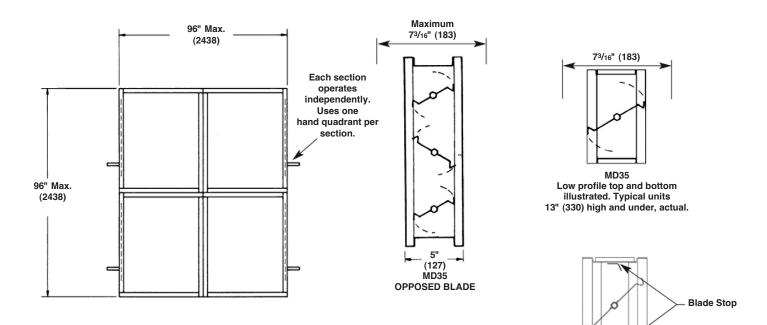
MD35 Blade Stop is standard for units 12" (305) high and under. Blade Stop is optional for units over 12" (305) high.
