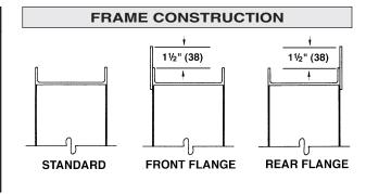
Dimensions in parenthesis ( ) indicate millimeters.
